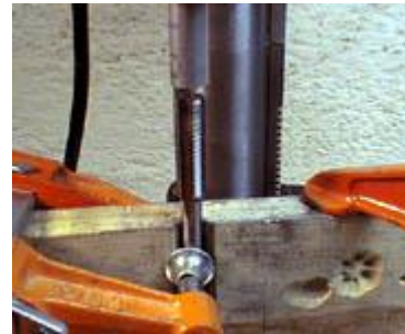
Tap the thread while the part is still in the chuck
