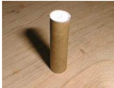
Finished grain ready for launch- note the kraft paper rolled on inhibitor/insulator
