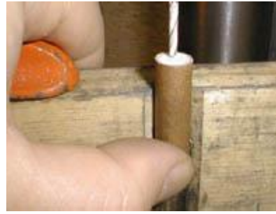
Drilling core in dextrose Bates grain
