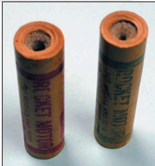
Early B16 and 1/2A motors. Note the thicker casings used in these old motors, and the larger nozzle diameter of the core-burning B16.
