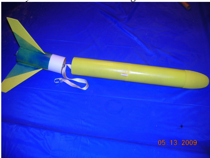
Glenn Roth's Big Yeller a dual egglofter design incorporating the "anti-zip feature."
